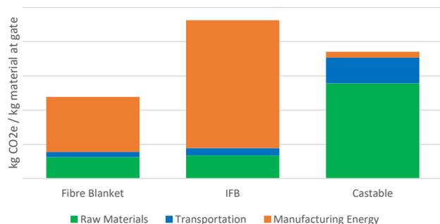
Fig. 2: relative climate change impact of various refractories as calculated by LCA (Cradle-to-Gate).
