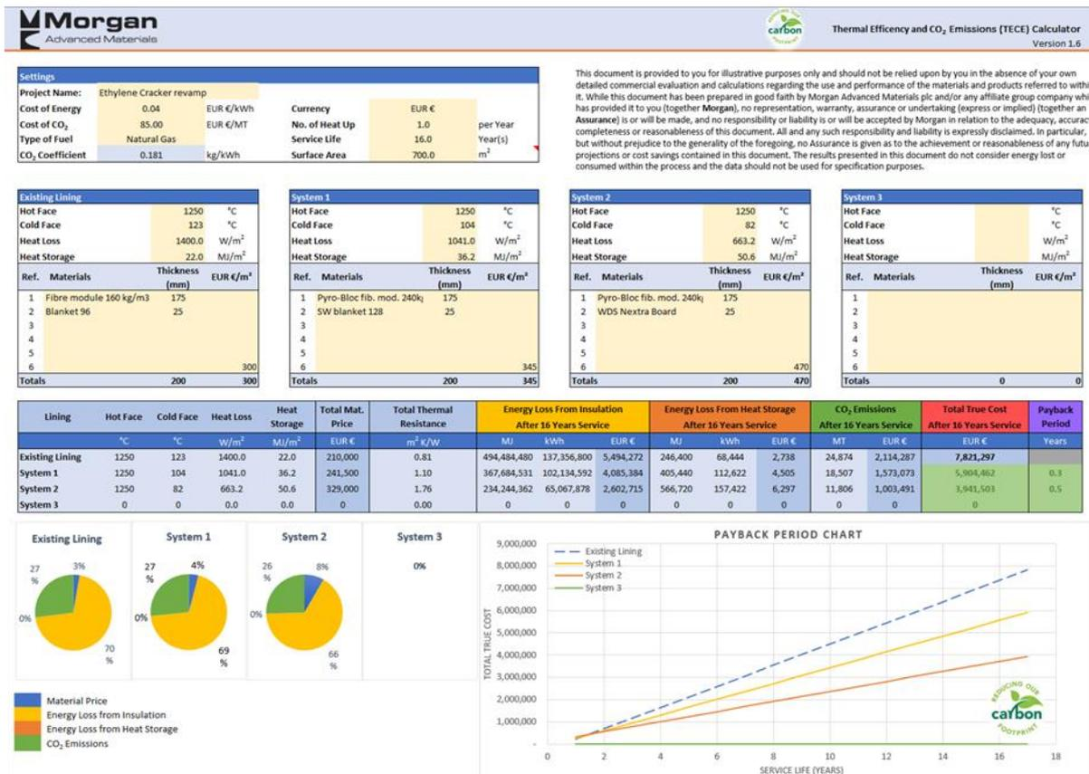
Fig 4 Thermal Efficiency and CO<sub>2</sub> Emissions (TECE) calculations for 3 alternative refractory linings for a 1250°C ethylene cracker walls
