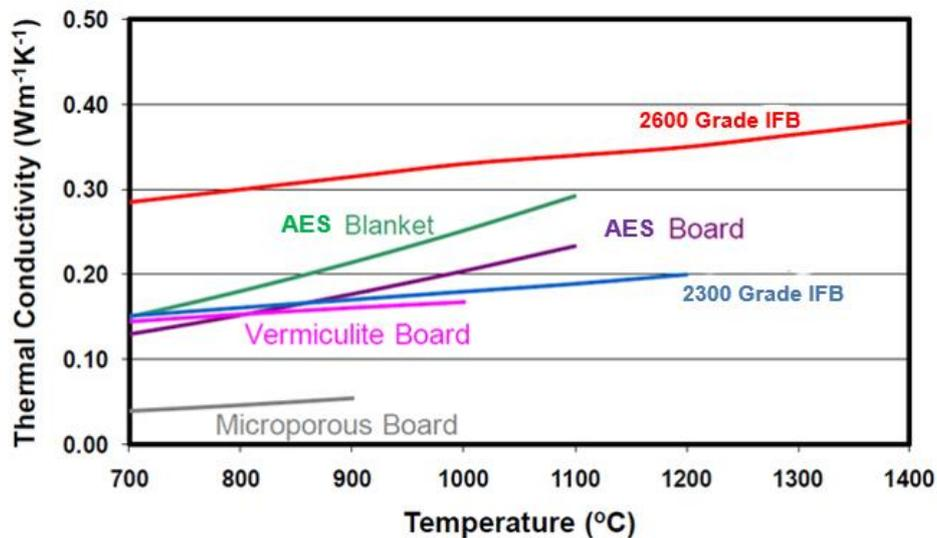
Figure 10: Thermal Conductivity across Common Refractory Product Line
