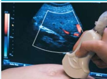
Technical Ceramics' piezoelectric materials produce a voltage proportional to applied mechanical pressure and, conversely, if a voltage is applied they change shape. Technical Ceramics uses these advanced materials to dramatically improve the performance of ultrasound transducers in medical applications, including sensors for catheters, blood pressure, vascular flow and medical imaging.
