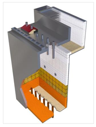
Ethylene Cracker – Sketch of radiant section
