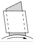
**Trailing** When the inclination of the brush centre line to the radial line is 'with' the rotation.
