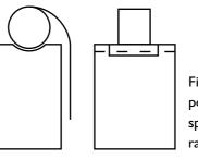
Fig. 10: Correct positioning of spring in top radius
