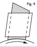
**Reaction** When the inclination of the brush centre line to the radial line is 'against' the rotation.
