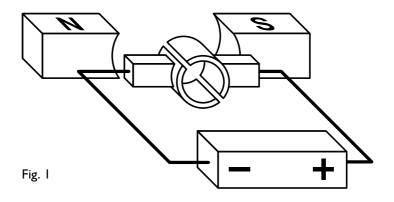
The carbon brush is the integral part on the transfer of current in the rotating machine and although they differ in size, shape and technical composition carbon brushes and collectors all fulfil the same basic function. This is to transfer current from a moving device to a stationary point or vice versa within an electric circuit.
