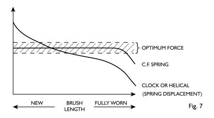
Traction motors generally represent an arduous test of brushes and brush holders because of vibration and the shock loads that the motors can receive. C.F. spring brush holders have generally proved to offer advantages over conventional spring brush holders in the traction applications, and large production orders have subsequently been received.
