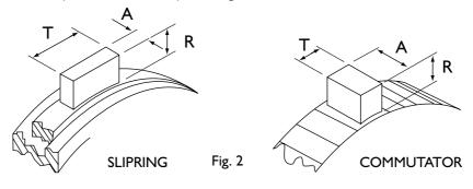
T = Tangential A = Axial R = Radial To the collector
