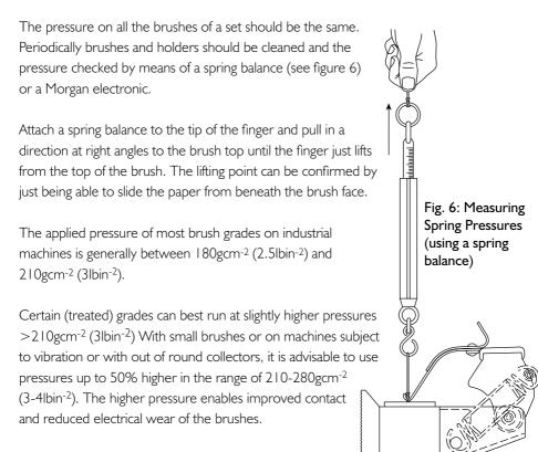
On traction motors, and on some fractional horsepower machines, higher pressures of 280-490gcm<sup>-2</sup> (4-7 lbin<sup>-2</sup>)
